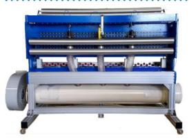
This is a **FAST AND STABLE DEVICE** designed to punch **MACRO HOLES** of various diameters and shapes in **MOVING MATERIAL** and in particular, it works with **PLAIN OR PRINTED FILM**. This model has to be integrated into existing machinery such as extruders, slitters, bag machines etc. It is suitable to make holes on fruits and vegetables bags, garbage bags, paper bags, foam etc.
